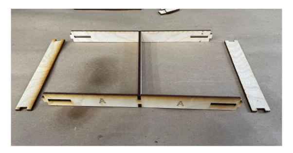
**Step 3**: Using 2 Unlabeled pieces, attach each one to the notches on both sides of the "A" pieces. This will complete the assembly of one of the frame inserts.
