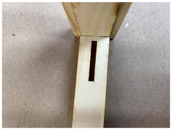
**Step 9**: Insert the 8 wedges into the eight slots. Be sure that they seat fully. (There should only be approximately 1/8" of the wedge exposed.)
